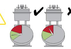
2 Prior to filling, check if more fuel is required by placing on the filling station. DO NOT refill an EcoBurner that is already full (at the top of the green area).
